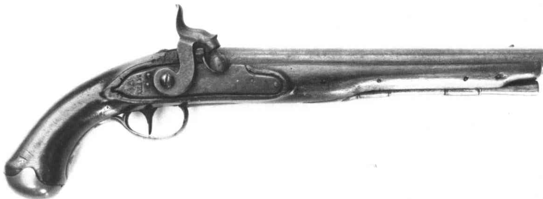
Third and last known Martin Fry 1808 pistol as altered to percussion. Fry delivered 116 pistols.
