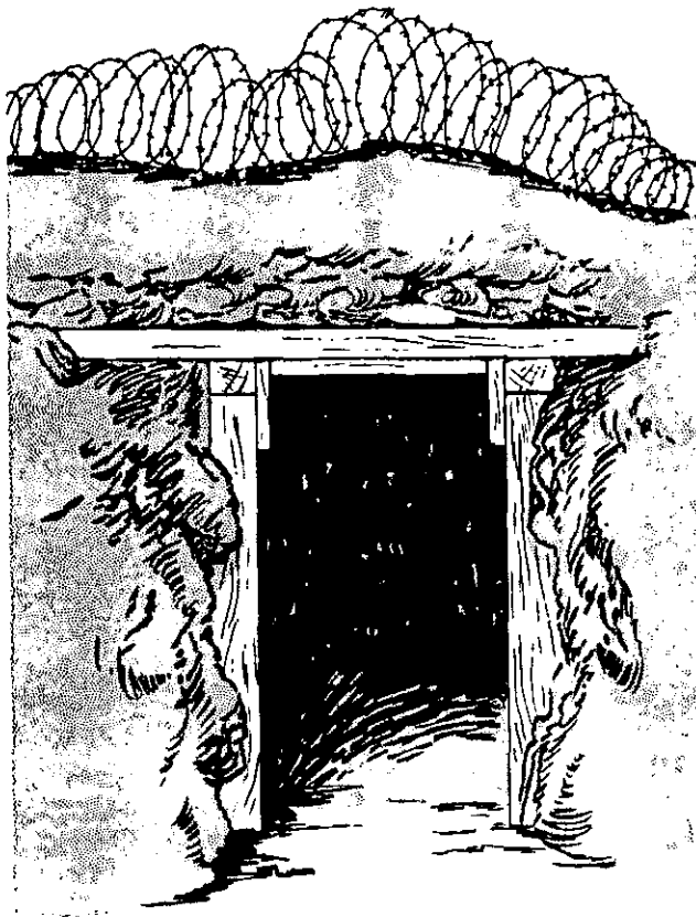
Figure 6-2. Protective wire on top of overhead cover.
