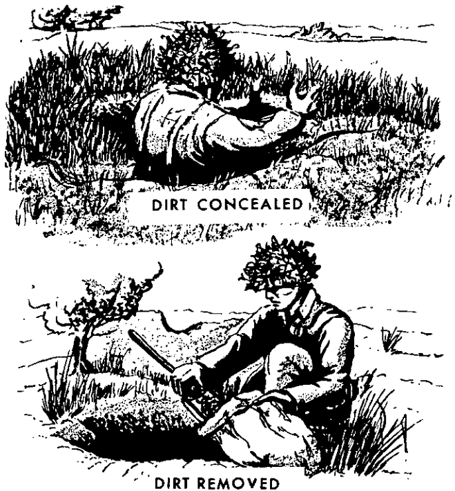
Figure 2-3. Disposal of soil.
