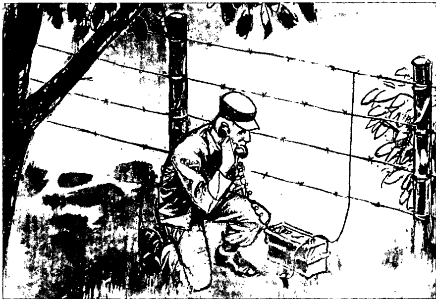
Figure 40. Expedient ground-return circuits.
