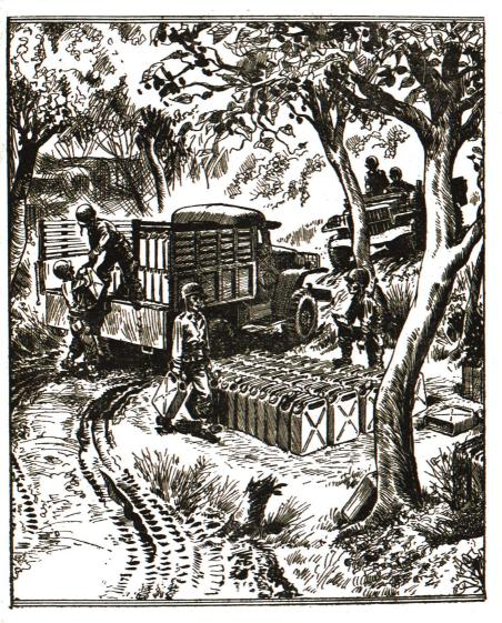
4. The cans should be farther off the trail, so that the loading truck can pull off and allow traffic to keep moving. This way, it is holding up the other truck, which incidentally is going the wrong way . . . one-way traffic in any dump is imperative.
