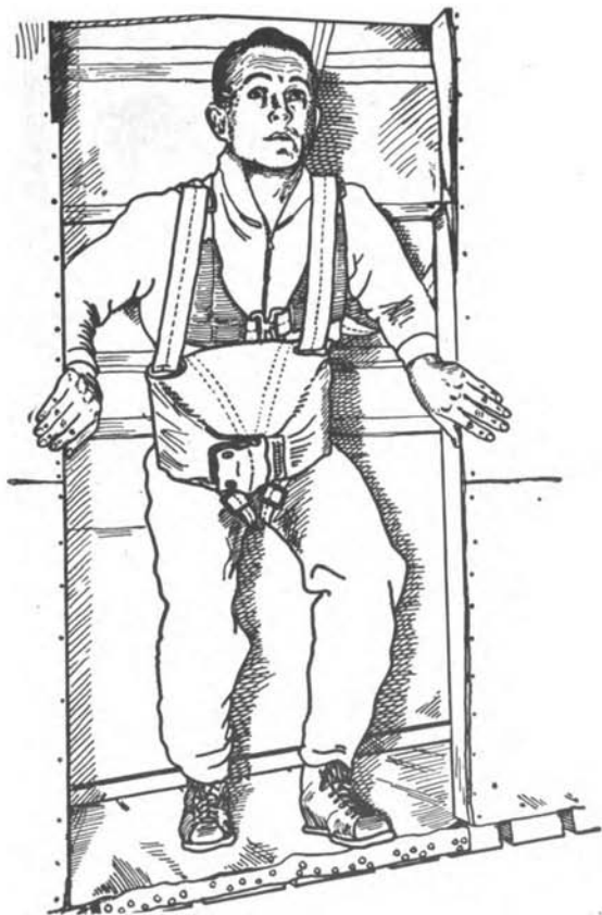
FIGURE 24. —Parachutist, wearing dummy parachute, in mock-up door of type C-33 airplane. Correct position for exit.
