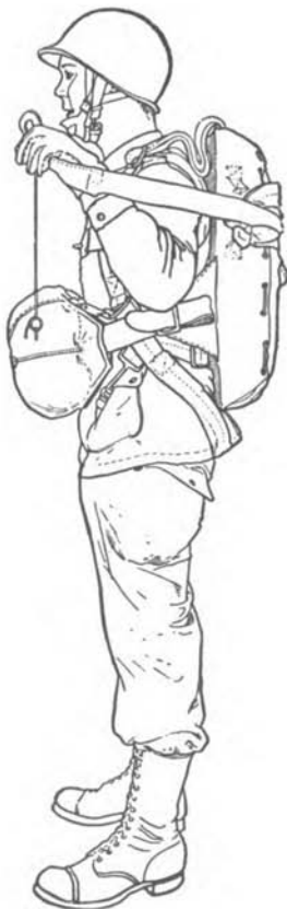
FIGURE 3. —Side view of individual parachutist, showing main canopy, pack on back, and reserve parachute on chest.
