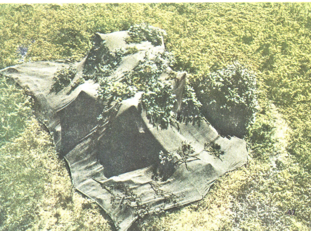
FIGURE 49 (c) and (d).—In upper picture, drape is unrolled over vehicle; ends are spread out and partially staked down. More of net is on the shady side, stretching out farther with a gradual slope. Draping must not stop at this stage. Below, poles prop net off top of vehicle, creating an irregular shape. Addition of small branches completes the job.
