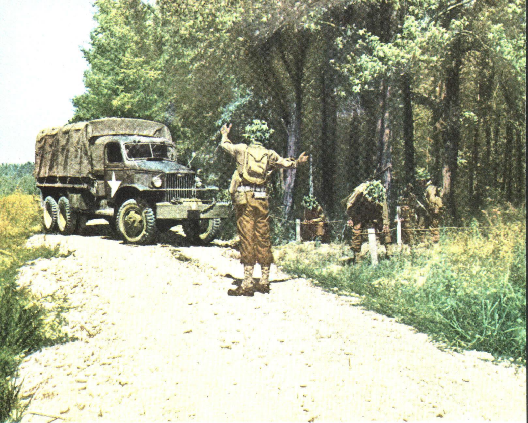
FIGURE 8.—Concealed entrance to a position. Route is wired in, and guides are posted to prevent changes in the appearance of the terrain.
