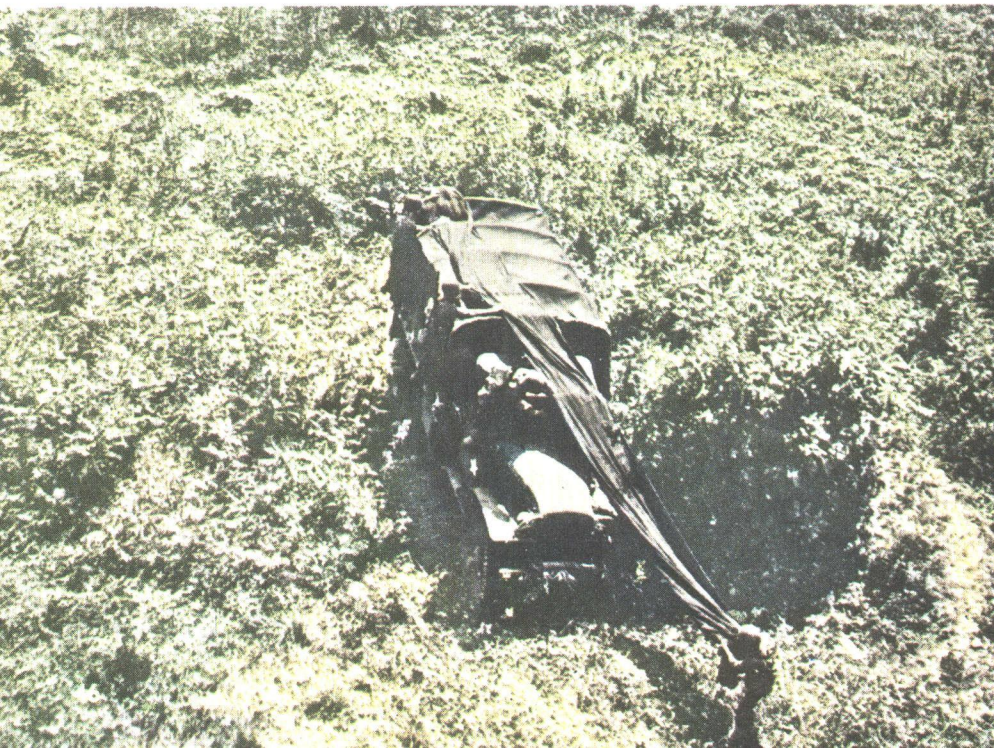
FIGURE 49 (a) and (b).—Steps in the erection of a drape. In upper picture, truck is parked close to bush. Reflecting surfaces which may shine are covered before the net is put on. Rear curtain is dropped to cover shadow in cargo space. In lower picture, net is unfolded so its long axis is diagonally over the truck and slightly off center.
