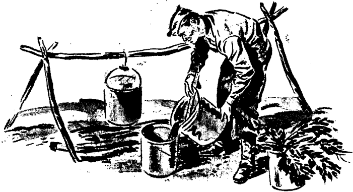
FIGURE 35. — Green vegetation being boiled in 5-gallon cans to make adhesive.
