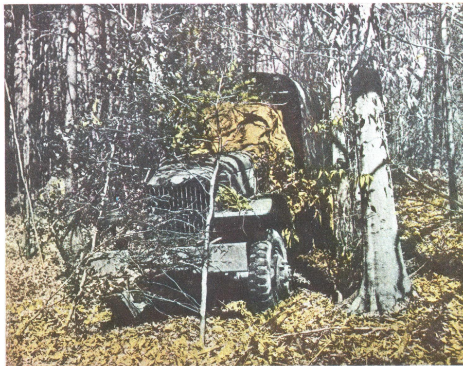
FIGURE 34.—A combination of natural materials and blankets prevents shine from headlights and windshield on this truck.
