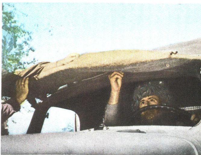
FIGURE 21. — The wise driver makes his own slip-on covers for headlights, windshields, and other reflecting surfaces. He keeps them covered at all times, if possible. They may be made of burlap, osnaburg, or salvage.
