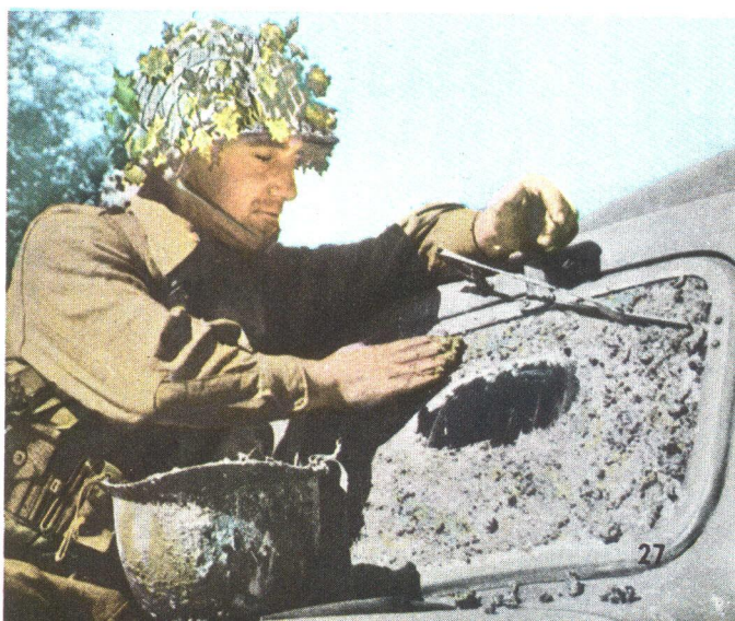
FIGURE 22. — Mud and leaves applied liberally to the windshield reduce shine. When moving, the area traversed by the windshield wiper should remain clear.
