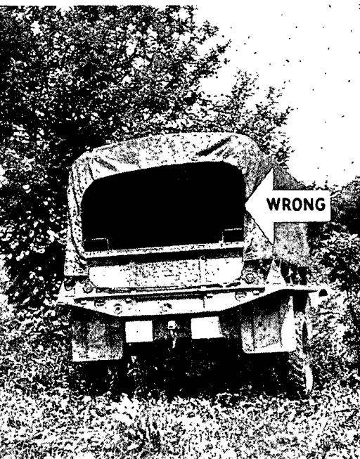
FIGURE 30 ① and ②.—The characteristic black shadow in the open end of a cargo truck can be seen for a considerable distance. One way to conceal this shadow is to drop the rear tarpaulin. Another way is to use natural materials, as shown here.
