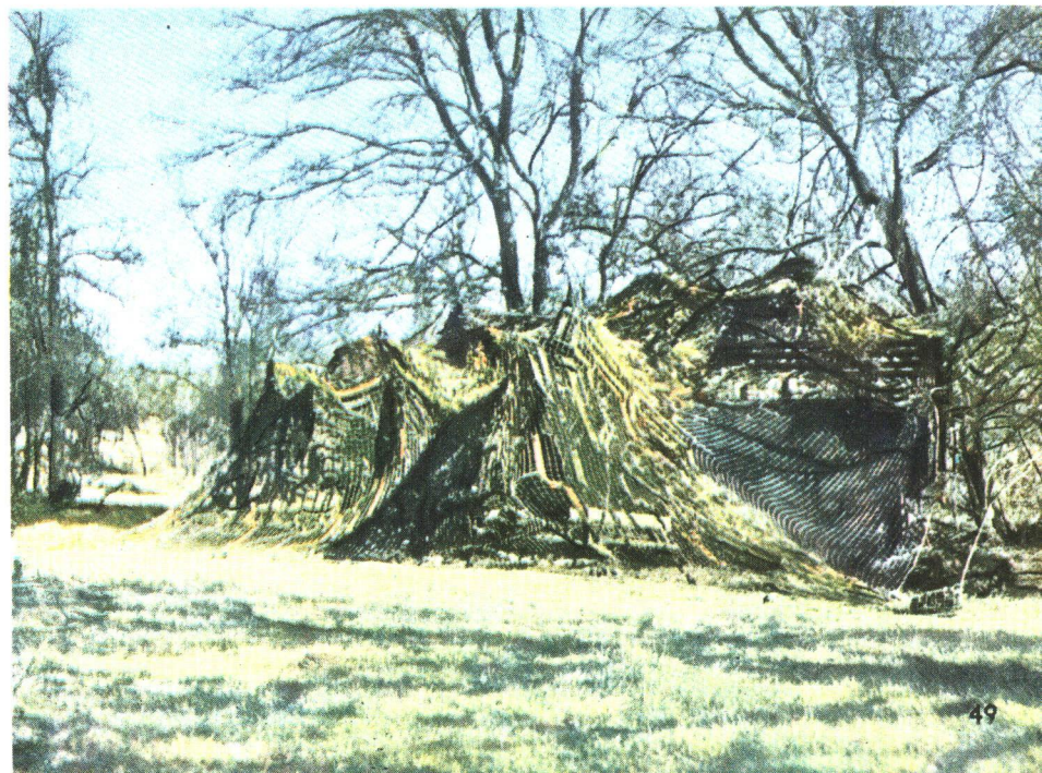
FIGURE 53.—Parked between two clumps of trees, this vehicle is draped with a well-propped net which joins the tree patterns.
