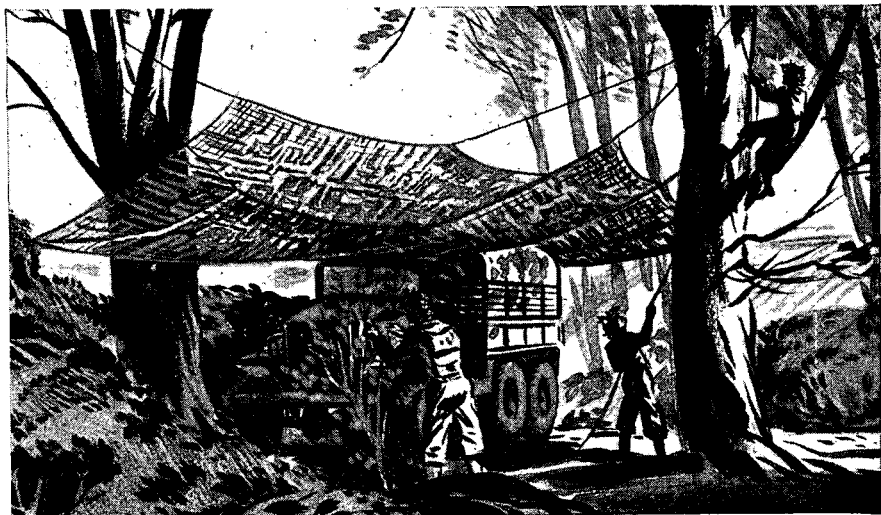
FIGURE 47.—An overhead screen provides good concealment. It is particularly valuable over more permanent parking places because it allows considerable freedom of movement underneath it and because vehicles can come and go while the camouflage remains in place. With this type of cover, a tight flat screen is unnecessary.
