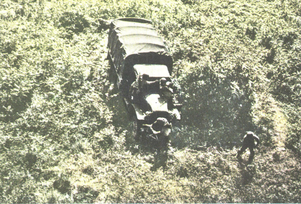
FIGURE 49 (a) and (b).—Steps in the erection of a drape. In upper picture, truck is parked close to bush. Reflecting surfaces which may shine are covered before the net is put on. Rear curtain is dropped to cover shadow in cargo space. In lower picture, net is unfolded so its long axis is diagonally over the truck and slightly off center.
