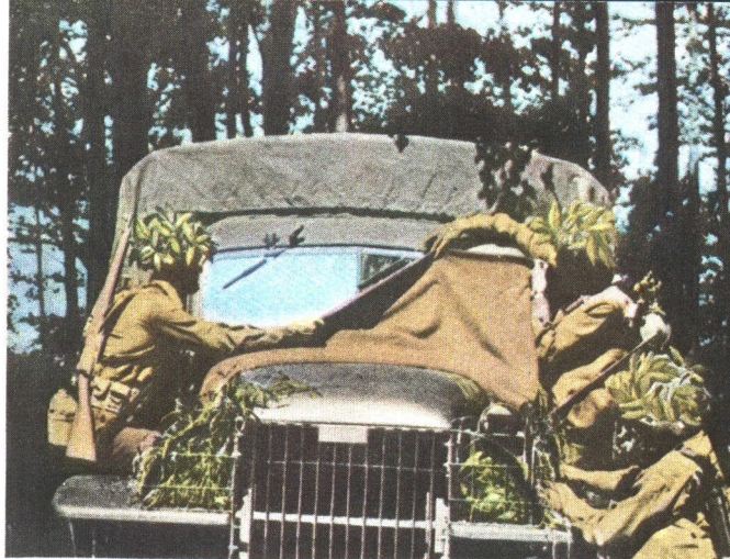
FIGURE 20. — Blankets, shelter halves, or pieces of dark-colored burlap or osnaburg are expedients for covering the reflecting surface of a windshield quickly. Foliage may be used to cover headlights.
