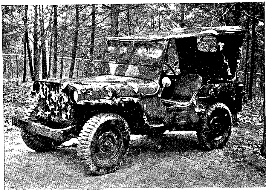
FIGURE 36.—Vehicle camouflaged with leaves applied with green-vegetation adhesive.
