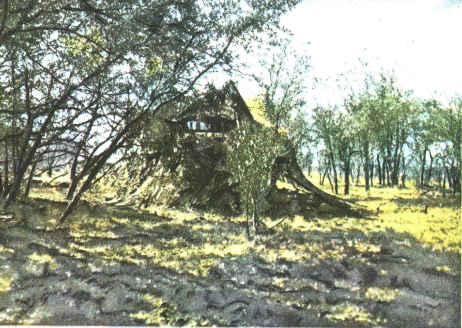
FIGURE 50.—Tank parked in shadow of tree. Garnished twine net, offset toward the clearing, ties the vehicle into the tree.
