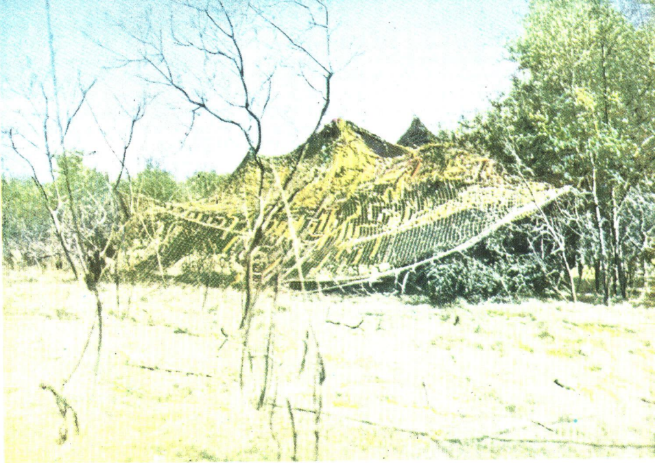
FIGURE 52.—A well-draped vehicle. Scrub has been used around the edges of the drape to break up the shadow made by the drape.
