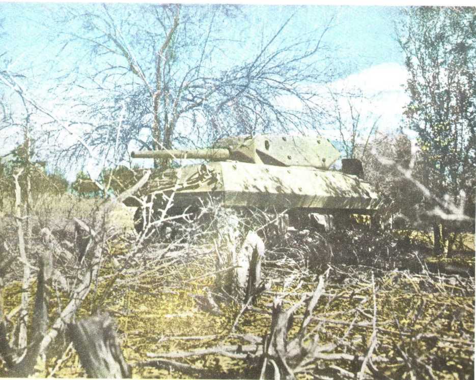
FIGURE 32.—Overhead cover is sparse here. This tank destroyer is sited so its over-all shadow is broken up. The long shadow line below the skirt is concealed from ground observation by natural materials.
