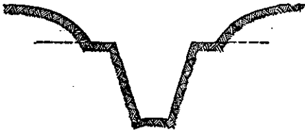
FIGURE 45.—Trench without flooring.
