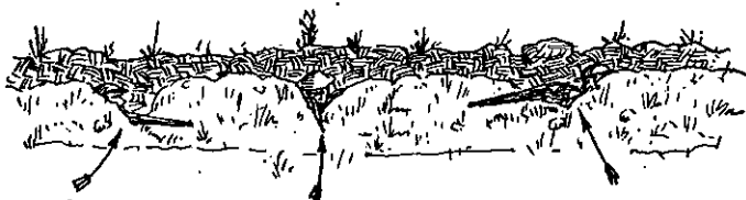
FIGURE 28.—Trench with irregular parapet and parados.
