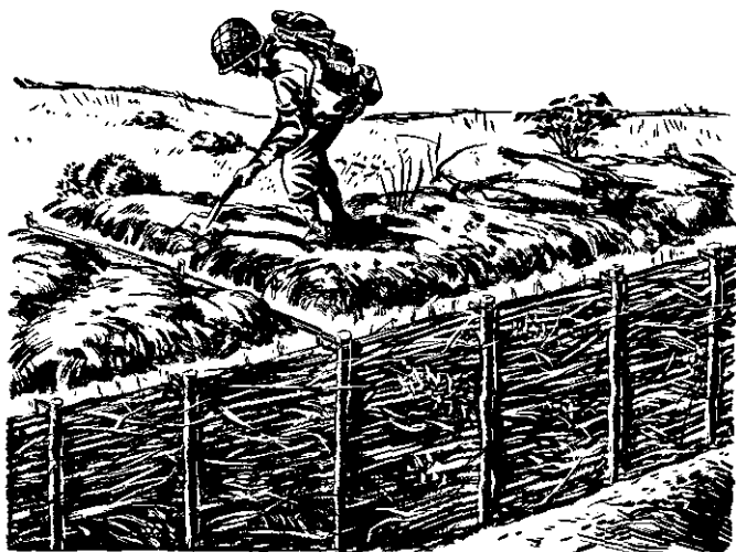
Figure 14. Continuous brush revetment.
