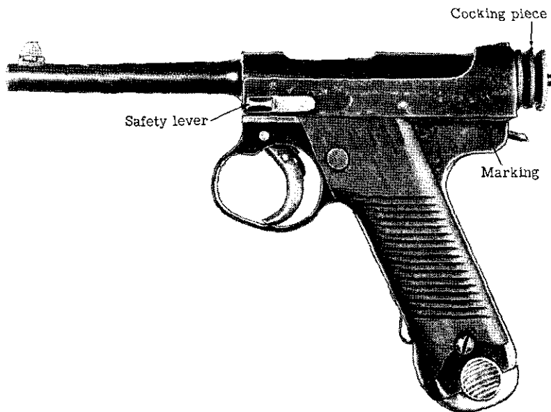
Figure 8.—Model 14 (1925) 8-mm pistol (left side).
