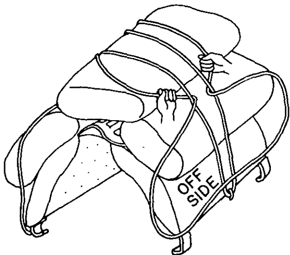
FIGURE 58. Pulling second loop out to form end ropes for top load (double diamond hitch).
