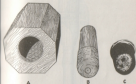
Figure 15. Punch and die used for straightening dented nose (right). A - Die, B - Punch, and C - Dented nose.
