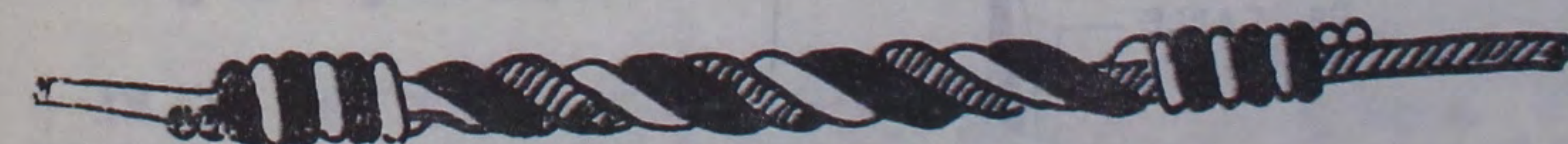
Fig 27.—Roll joint with binding wire
