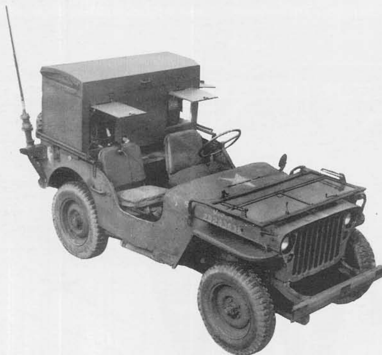
1. Radio Transmitter BC-902-B 2. Radio Set SCR-610-A 3. Power Unit PE-88 4. Shelter S-2/MRN-3 5. Roll BG-56
