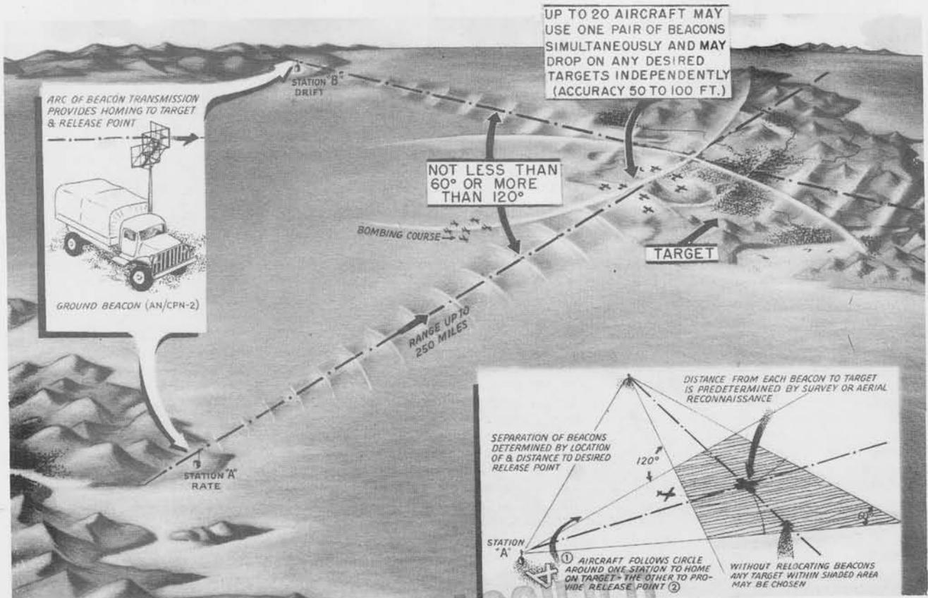
Radio set AN/APN-3 is the airborne element of an Aircraft Navigation System employing radar ranging and principles known as SHORAN. It may be used for precision bombing, dropping paratroops and supplies, aerial mapping, or precision navigation of aircraft and surface vessels.
