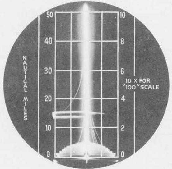
Scope records range vertically on three scales & azimuth horizontally right or left of centerline of Beacon Response signal; above shows simulated beacon 33 miles away and approx. 30° right.
