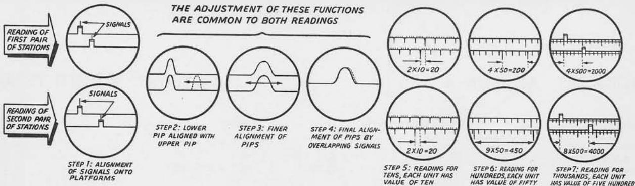
Radio Set \*AN/APN-4 is the airborne receiver element of the Loran Navigation System with which a radar fix is obtained by taking a reading on each of two Loran chains in the order shown.
