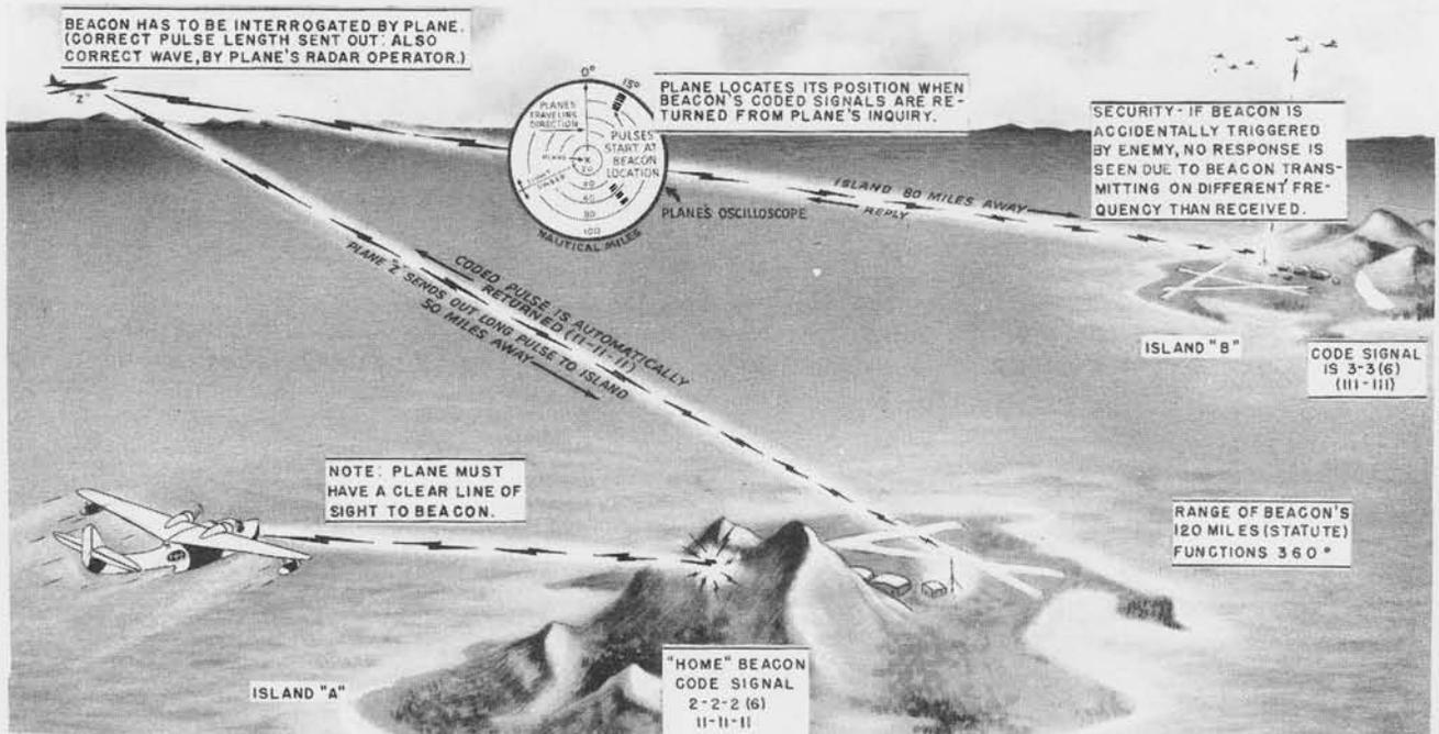
Radio Set AN/CPN-3 is an air transportable radar beacon designed to provide range, direction and identification for the homing of 10 cm band ASV radar equipped aircraft.
