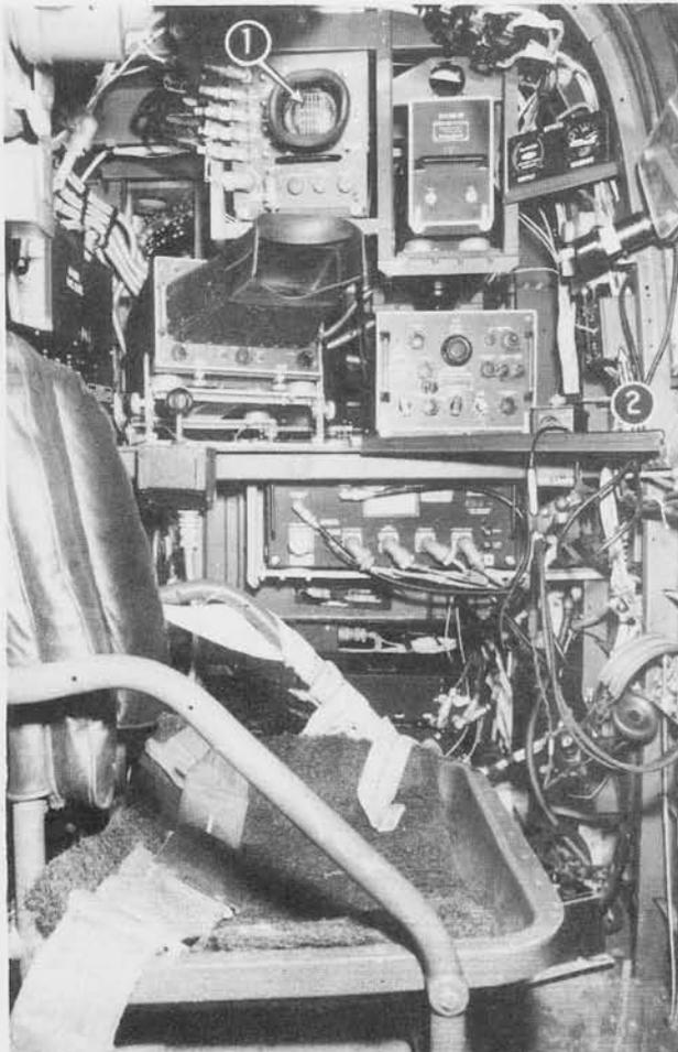
(1) Indicator BC-929-A (2) Radio Control Box BC-1145-A
