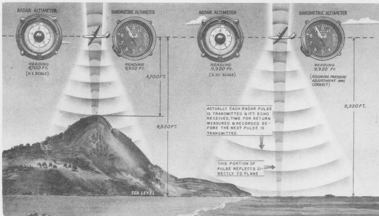
Radio Set SCR-718 is a precision altimeter which records the absolute altitude of an aircraft above the terrain, regardless of air pressure or variations in temperature.
