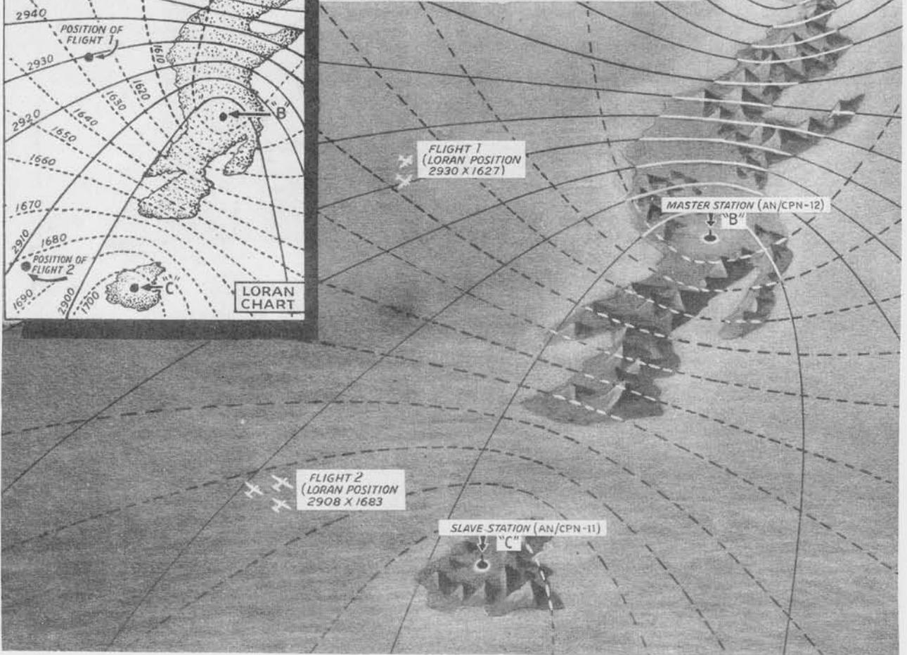
Radar Sets AN/CPN-11 and AN/CPN-12 constitute an air transportable ground Loran chain which provides properly equipped aircraft with means whereby they may obtain a fix of position at any time within the range of 200 miles by day and 400 miles at night.
