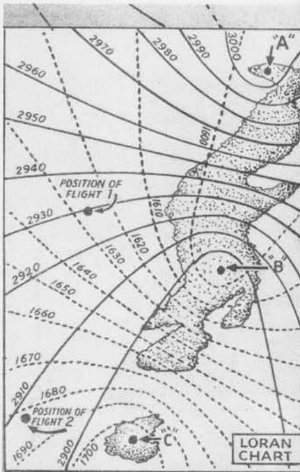
TO ESTABLISH POSITION THE AIRCRAFT TAKES BEARING ON ONE OF TWO LORAN CHAINS (A+B) WHICH ESTABLISHES AIRCRAFT'S LINE OF POSITION— (A HYPERBOLIC CURVE DRAWN THROUGH ALL POINTS WHOSE DISTANCES FROM THE TWO TRANSMITTERS OF THAT CHAIN ARE PROPORTIONATE (SEE CHART, LEFT)... TO GET EXACT POSITION (FIX) ON THIS HYPERBOLA THE AIRCRAFT TAKES BEARING ON THE SECOND LORAN CHAIN (B+C) WHOSE HYPERBOLAS CROSS THOSE OF THE FIRST.
