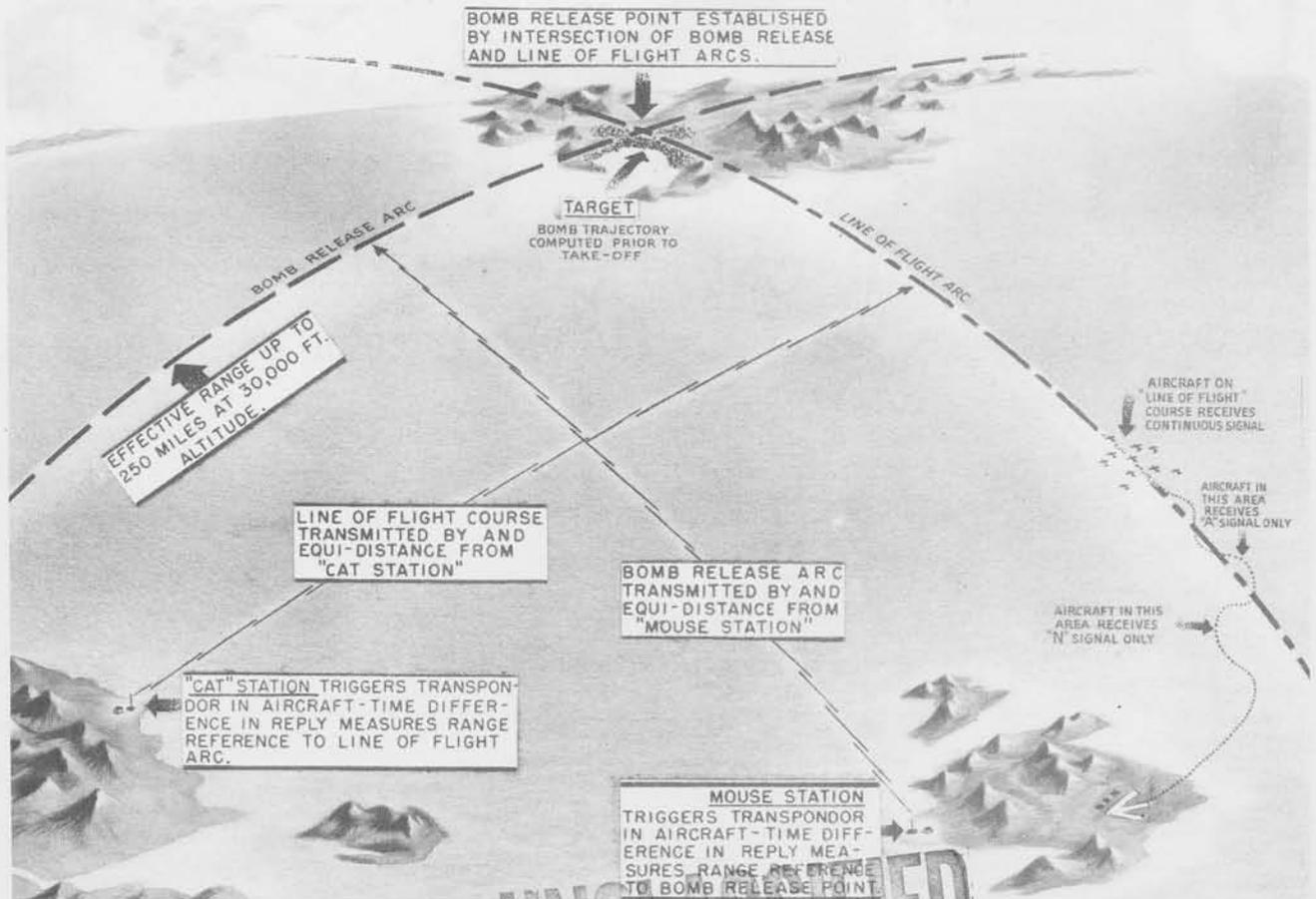
Radar Assembly AN/APA-9 ("ASPEN") is the airborne element of the OBOE Navigation System which in addition to facilitating precision blind bombing - may be used as a navigation device to direct reconnaissance or troop carrying aircraft to predetermined areas.
