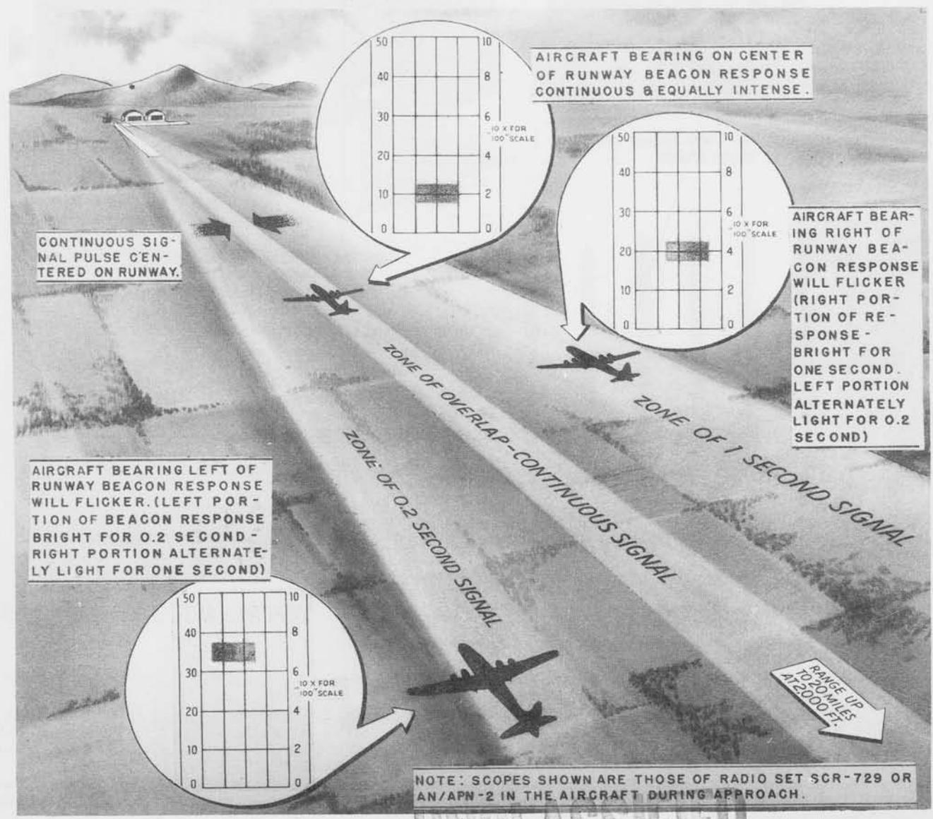
Radio Set AN/CPN-7 (BABS) is air transportable radar beacon transponder which provides means of landing aircraft equipped with Radio Set SCR-729 or Radio Set AN/APN-2
