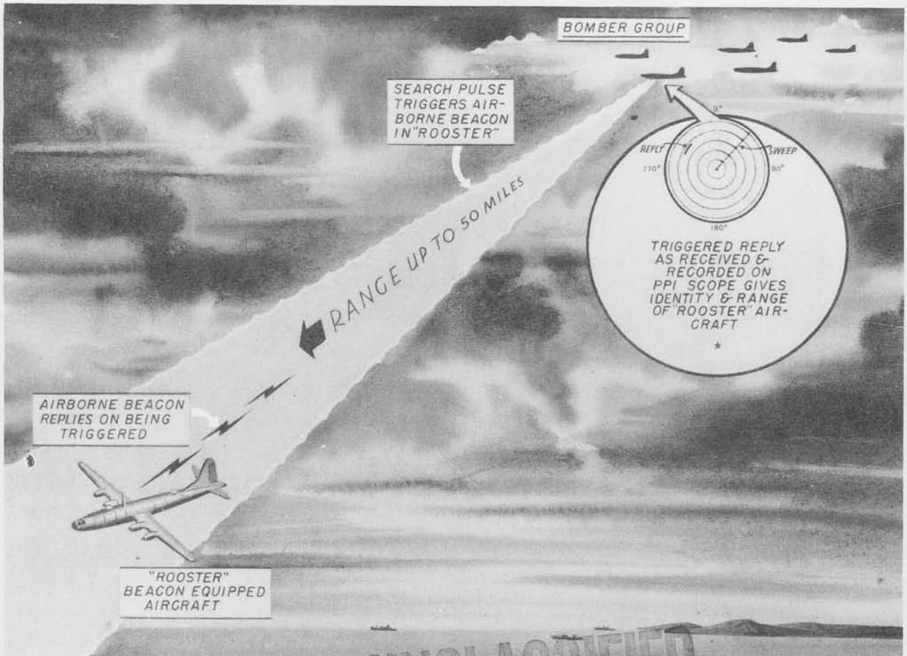
Radar Beacon AN/APN-7 is an airborne transponder beacon used to establish the identity of the aircraft in which it is installed and provide navigational aid to other aircraft.
