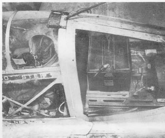
Radio Set SCR-522 installed in P-38E aft of pilot position
