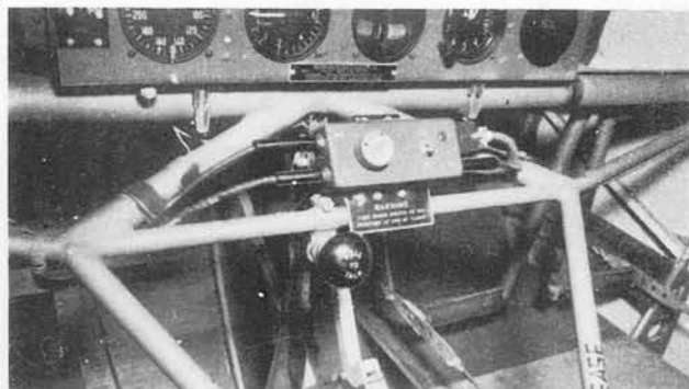
Installation of Control Box and "pull to talk" switch on instrument panel, pilots position in CG-4A glider.
