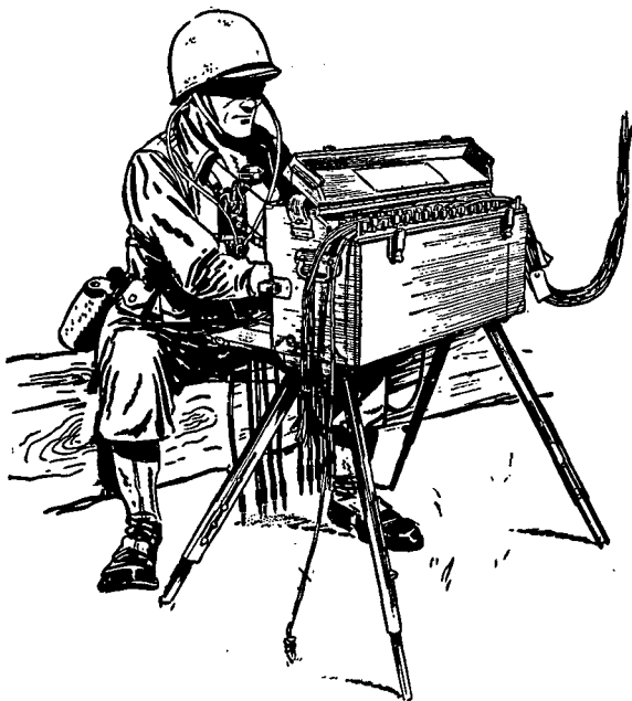
Figure 78. Switchboard BD-72 set up for operation, showing terminal compartment open.
