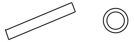
Tent Pole coupler/ sleeve made from water pipe or a Fence Pole coupler – .6 inch up to 1. Ft, .6 inch in length – depending on size and length of tent pole. Water pipe or Fence Pole couplers should be available at most Home Improvement or Hardware stores. You will need to fit coupler to your desired pole stock. Coupler will be slightly bigger at outside circumference to pole stock and slightly smaller at inside circumference than pole stock.
