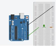
2) **Wire the Yellow LED:** Place the yellow LED, 1 resistor, and 2 jumper wires according to the diagram below. In this diagram the yellow wire is connected from the same row as the yellow LED to the digital pin 4 on the Arduino. The positive, or longer leg, of the LED should be towards the wire and the negative, or shorter leg, of the LED should be towards the resistor.
