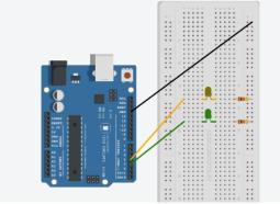
3) Wire the Red LED: Place the red LED, 1 resistor, and 2 jumper wires according to the diagram below. In this diagram the red wire is connected from the same row as the red LED to
